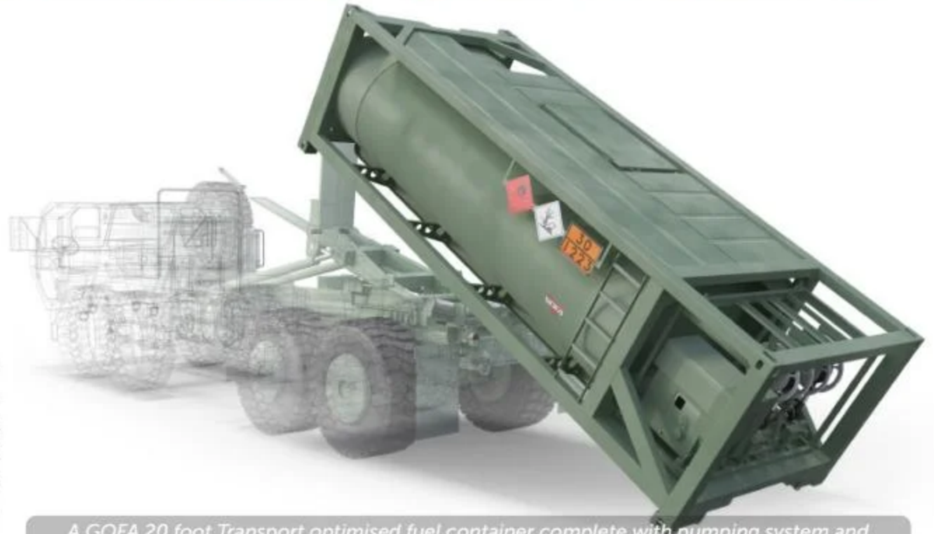
A GOFA 20 foot Transport optimised fuel container complete with pumping system and its own generator and fitted with a hook arm. The design is based on the standard ISO frame which enables it to be moved intermodally throughout the supply chain.
